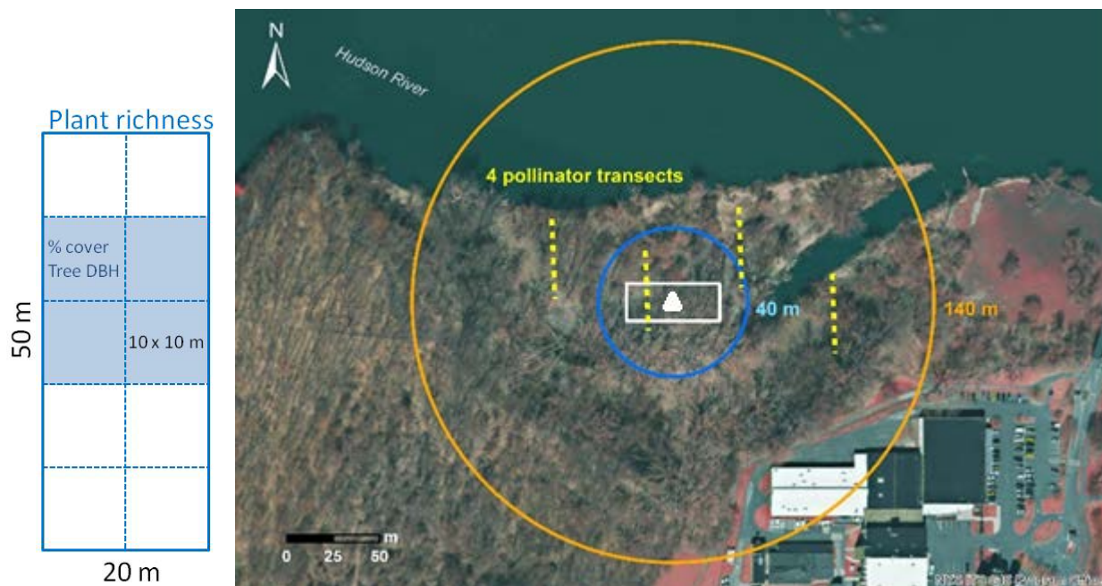
Figure 1: Left – schematic of the 20 m x 50 m macroplot. Right - Example placement of an East-West macroplot (white rectangle), centered around a random point (white triangle). That is, the point is the 25 m mark of the macroplot. At this site, 0 m is at the western end of the macroplot and 50 m is at the eastern end. Blue and orange circles represent survey areas covered during the Rapid Assessment Method survey(s). This figure also demonstrates how pollinator bowl transects may be laid when completing the intensive Empire State Native Pollinator Survey protocols (i.e., four transects within the wetland habitat); Note: pollinator transects do not need to be placed parallel nor are they likely to be perfectly spaced. Pollinator sampling is not part of our standard wetland assessment sampling protocols.
