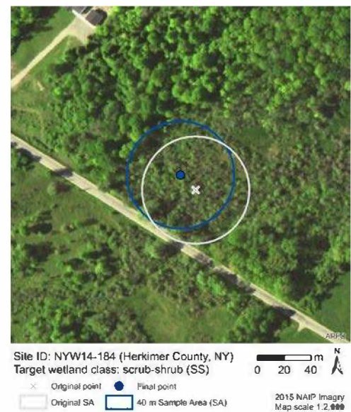
Figure 31: Sample Area around original random point included a road and some forested area ( >10\% non-target), so the point was moved \sim 15 m northwest
